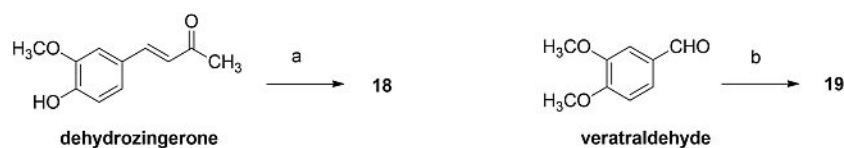
Scheme 3. compound 18 : (a) 2,3,4,6-tetra- O -acetyl- \alpha -D-glucopyranosyl bromide, \text{Ag}_2\text{CO}_3 at rt in pyridine for 18 h, then, after purification of the product, \text{CH}_3\text{OH}/\text{CH}_3\text{ONa} solution at rt for 10 min; compound 19 : (b) per-O -acetylated- \beta -D-glucopyranosyl ketone, pyrrolidine at rt in \text{CH}_2\text{Cl}_2 , 72 h, then, after purification of the product, \text{MeOH}/\text{MeONa} at rt for 10 min.
